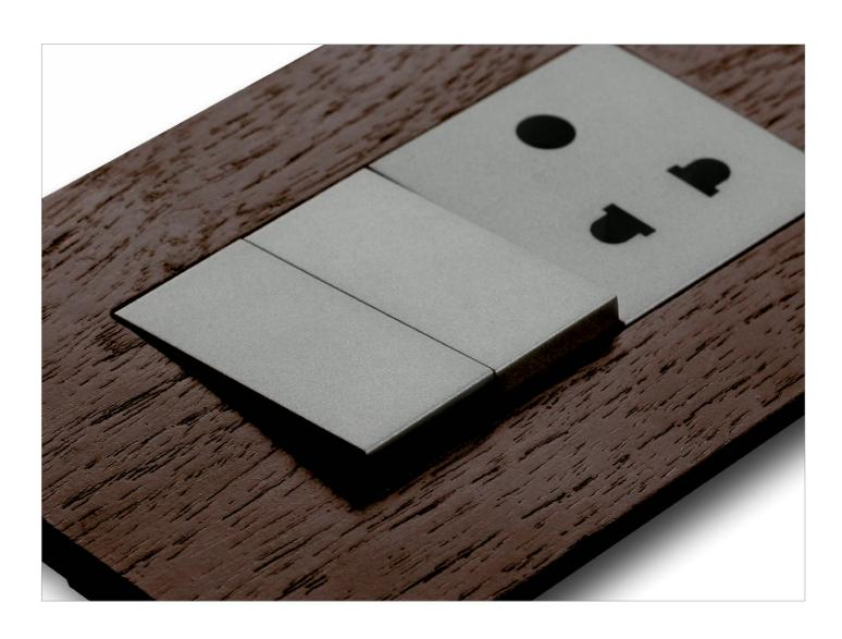
CUBE Series switches have contacts which provide very high current carrying capacity. The contact design, snap action mechanism, appropriate contact pressure, wiping action between the contacts and use of high engineering grade materials result in minimum arcing. Reduction in arcing ensures a very long operating life for the switches.
